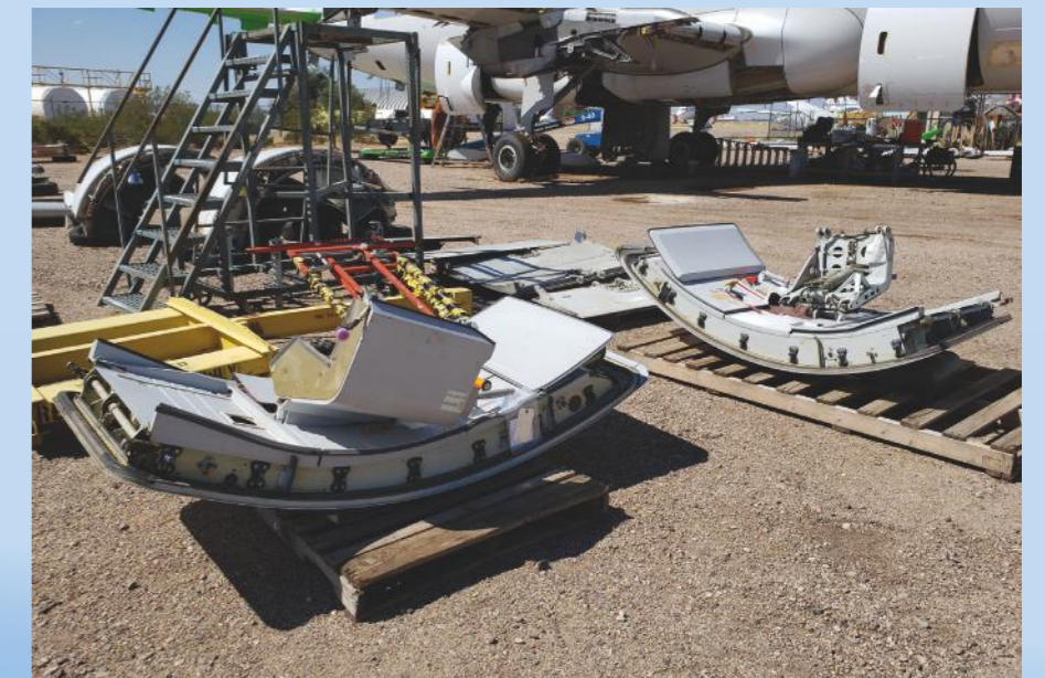
Parts identification tags are attached to all parts following removal and cleaning
